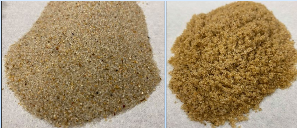
Photos of water-wet (left) and oil-wet proppants (right).
