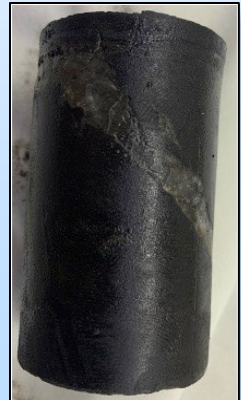
The mudstone Cane Creek sample contains a 7 mm thick natural fracture filled with migrated salt.
