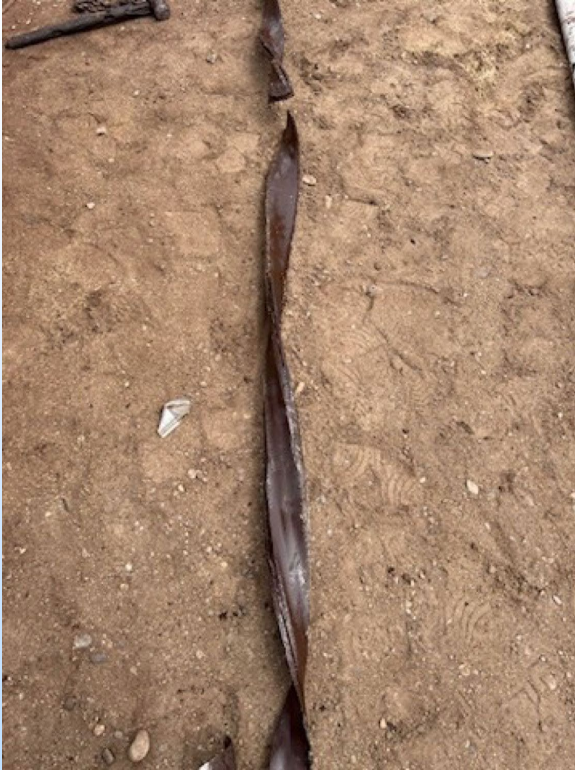
Twisted 2 7/8" tubing recently removed from the hole
