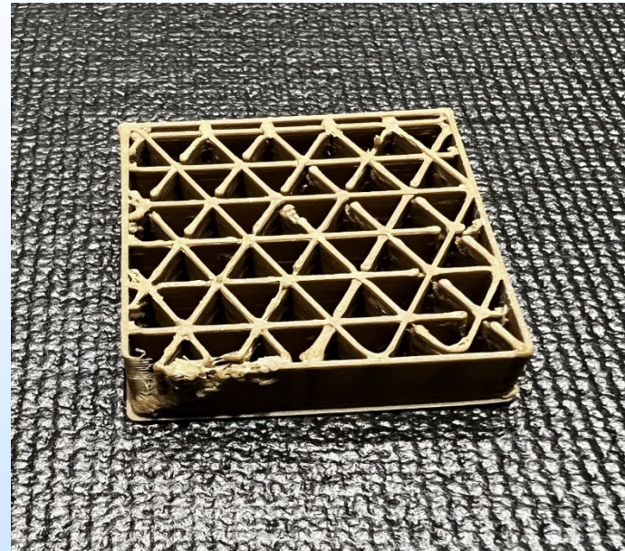
A small part made from 50% coated fly ash in polypropylene.
