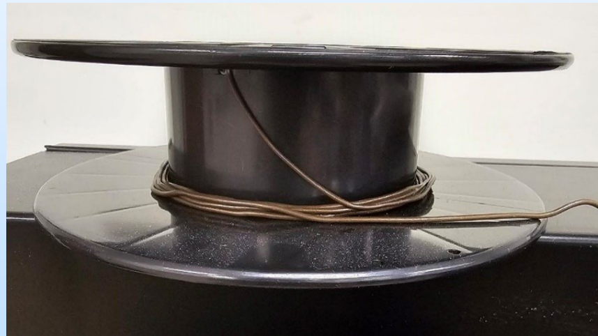
Filament (1.5mm dia.) produced using B235 and lignite fly ash.
