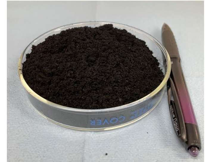
Photograph of ~ 3.0 g of 3DG-900 in 100 mL petri dish (tap density ~0.035 g/cm 3 )
