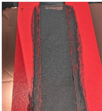
Figure 9: Tape cast anode from coal char hard carbon.
