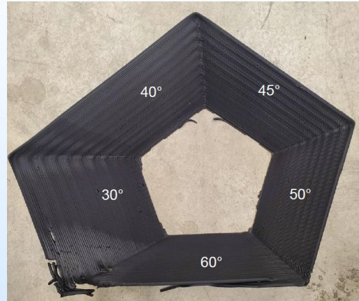
Positive overhang test (2 mm nozzle)
