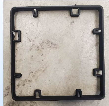
Bridge test (2 mm nozzle)
