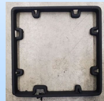
Bridge test (4 mm nozzle)
