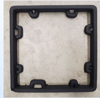
Bridge test (6 mm nozzle)
