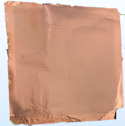
Coal-derived Graphene coated on C110 at 40 °C using UC
