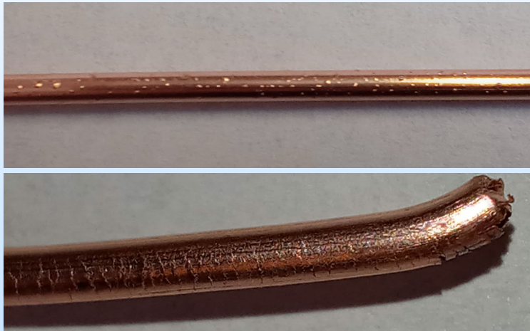
CMC starts with blisters and some cracking
