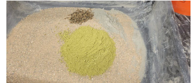
Above: Concrete mix ingredients (sand, leached CFA, cement, and gravel)
