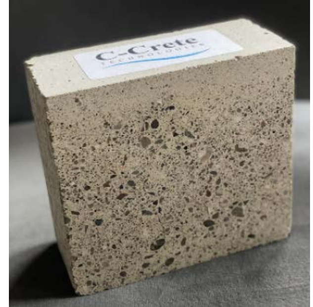
Sand blasted (Terrazzo floor)
