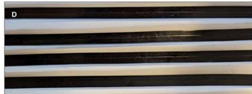
A. Reza holding an 80 wt.% filler ShAPE composite extrudate; B. Tooling cavity designed for manufacturing composite 'bars'; C. Cold-pressed composite feedstock granules in ShAPE ring; D. ShAPE polymer composite bars with no surface defects
