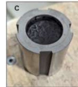
A. Reza holding an 80 wt.% filler ShAPE composite extrudate; B. Tooling cavity designed for manufacturing composite 'bars'; C. Cold-pressed composite feedstock granules in ShAPE ring; D. ShAPE polymer composite bars with no surface defects
