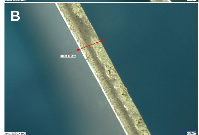
Figure above shows optical micrograph at 100X magnification of EEA sample prepared at 90 °C through A) 1 pass calendering with a set gap of 330.2 um, where 2 individual ASL green sheets were laminated onto a double-layer coated green sheet of AFL/GDC resulting in a 9.0% reduction in thickness to 252 um from 277 um. B) 2 pass calendering, first of the GDC onto the AFL followed by addition of 2 ASL layers onto the assembly, laminating at a set gap of 457.2 um. The initial thickness of 380 um was compressed by 9.7% down to 343 um.
