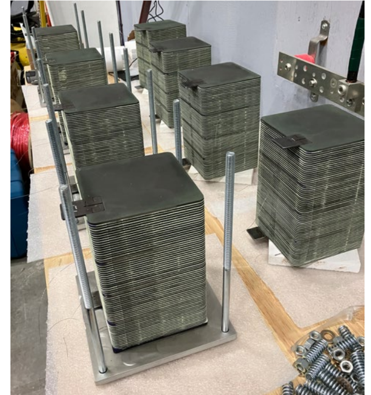
OxEon stacks being prepped for installation
