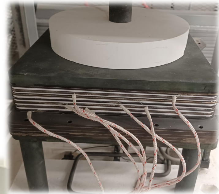
1 kW SOEC stacks with 300 cm 2 active area cells
