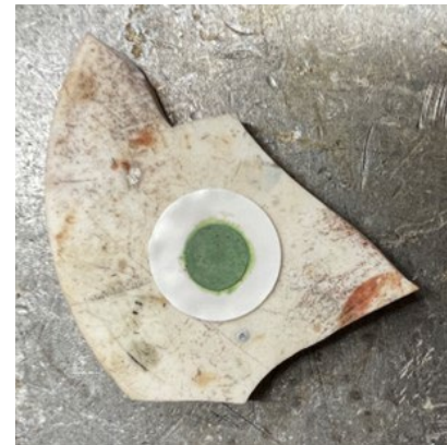
Anode infiltrated with \text{Ni}(\text{NO}_3)_3 solution and heated to 1300\text{ }^\circ\text{C}
