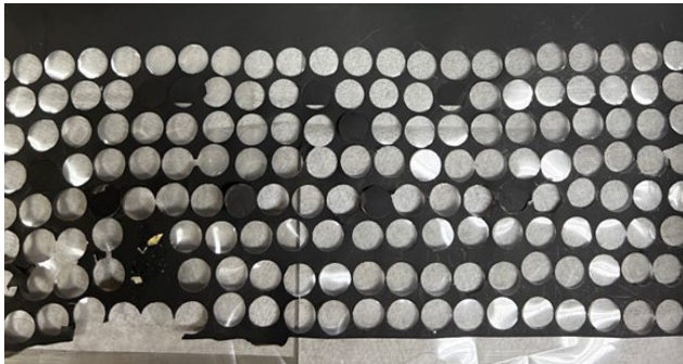
YSZ tape with graphite pore former used for making electrode layers
