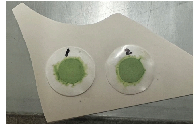
Cell infiltrated by Ni(NO_3)_3 on the anode side and heated up to 1100 °C
