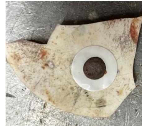
Cathode infiltrated with LSF solution followed by drying.
