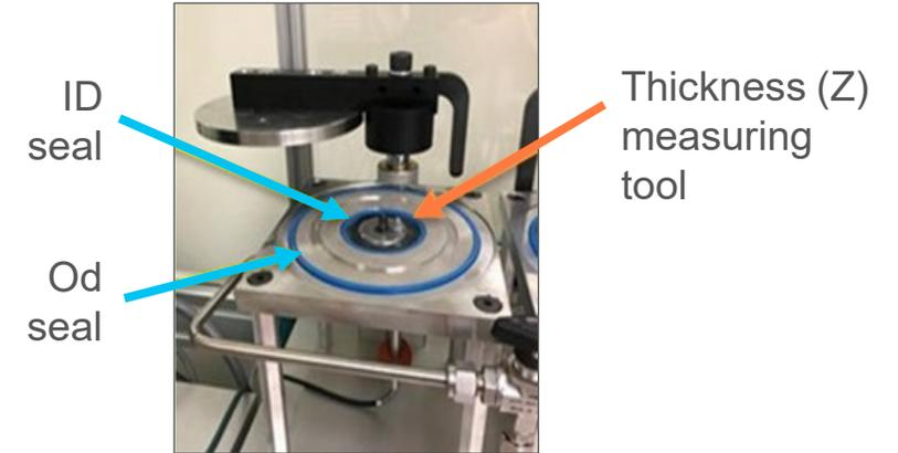
CSA cell leak tester jig with thickness measuring tool
