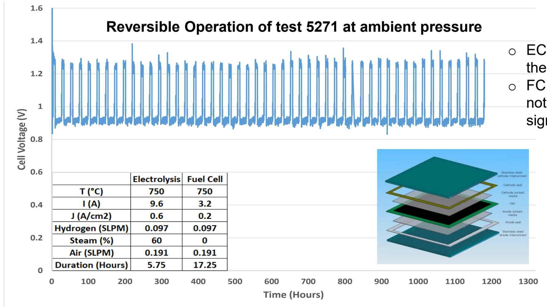
**Reversible operation of a 16 cm<sup>2</sup> cell at ambient pressure (46 SOEC/SOFC cycles over 1,104 hours)**
