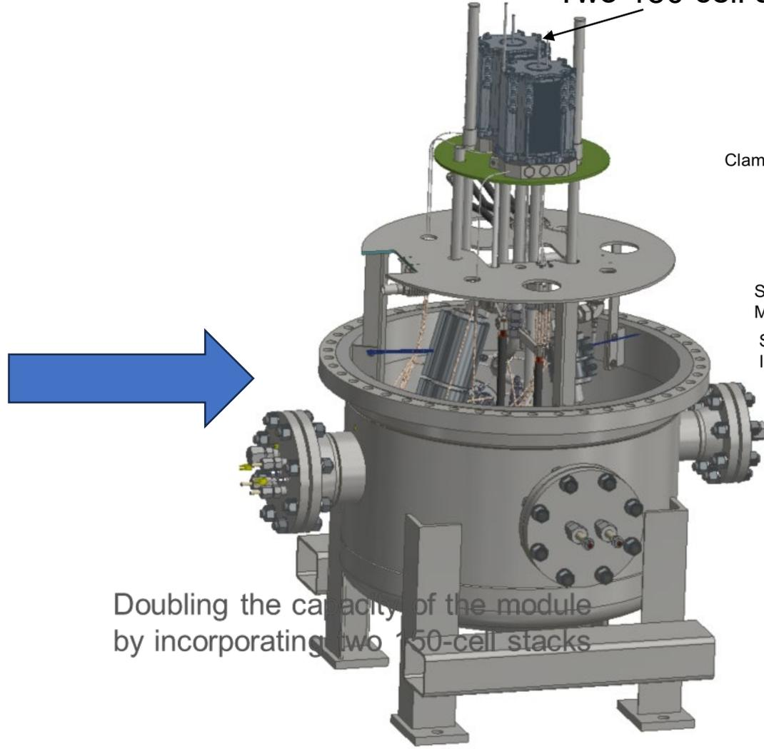
Doubling the capacity of the module by incorporating two 150-cell stacks
