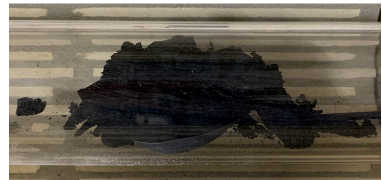
Post-decomposition structured catalyst/support disk
