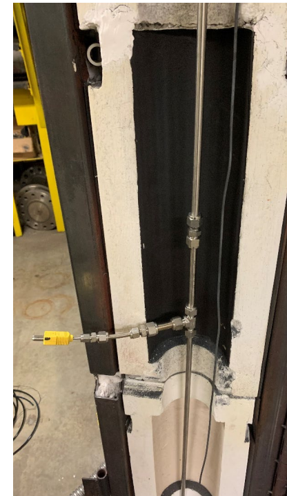
Fluidized/Fixed bed testing in 3/8-inch tube reactor
