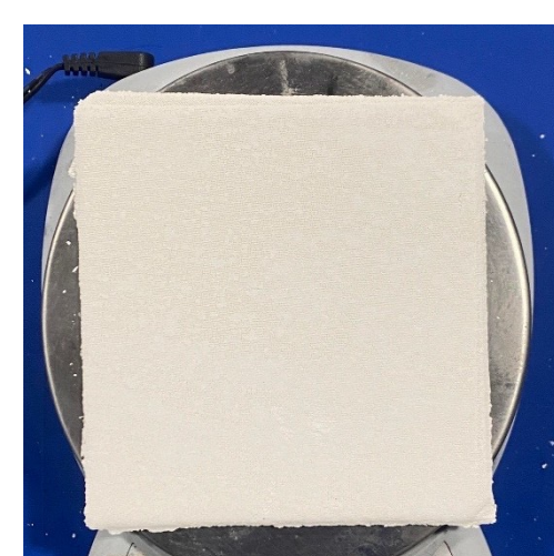
The 'preform' is dried in autoclave for 2 hours at 180°C
