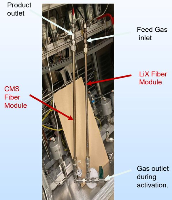
Additional LiX packed in a few 2<sup>nd</sup>-layer dual-modules to adjust N<sub>2</sub> removal.
