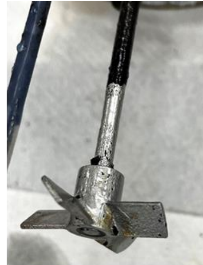
Corrosion on stirrer (left) and aqueous fraction (right) from acidic conditions
