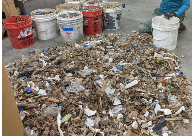
Figure 3 C&D waste shear-shredded to 2" minus and screened for metals, preparing for hammermilling
