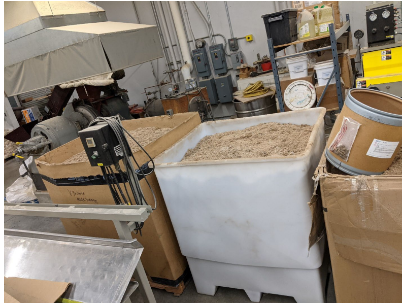
Figure 5 Hammermilled C&D waste "fluff," preparing to be pelletized
