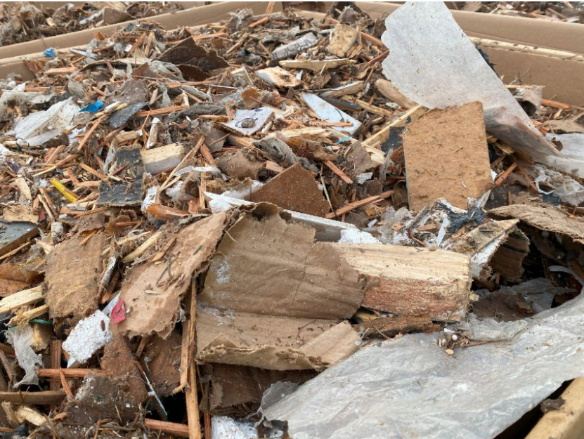
Figure 2 C&D waste shear-shredded to 4" minus and screened for ferrous and non-ferrous metals in a car shredder
