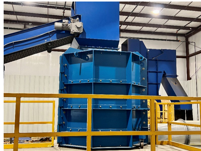
Vertical Shaft Impactor (dewatering and size reduction unit operation)
