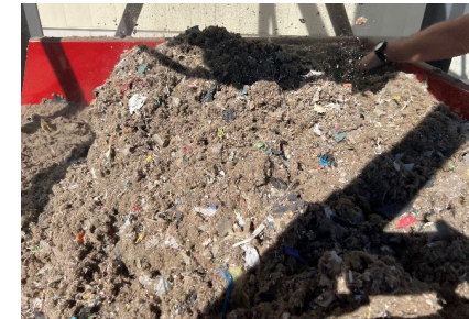
RDF Fluff (Processed MSW)
