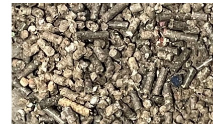
Pelletized RDF (easy to transport and feed)
