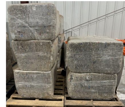
Baled RDF (plastic wrap seal enables excellent long-term storage)
