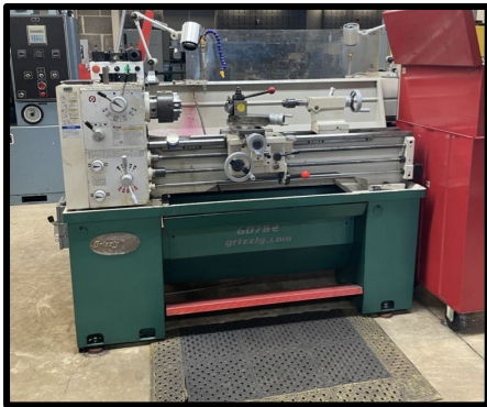
Grizzly G0782 – 13” x 40” Gearhead Lathe
