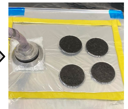
This 'densifies' the composite and reduces porosity
