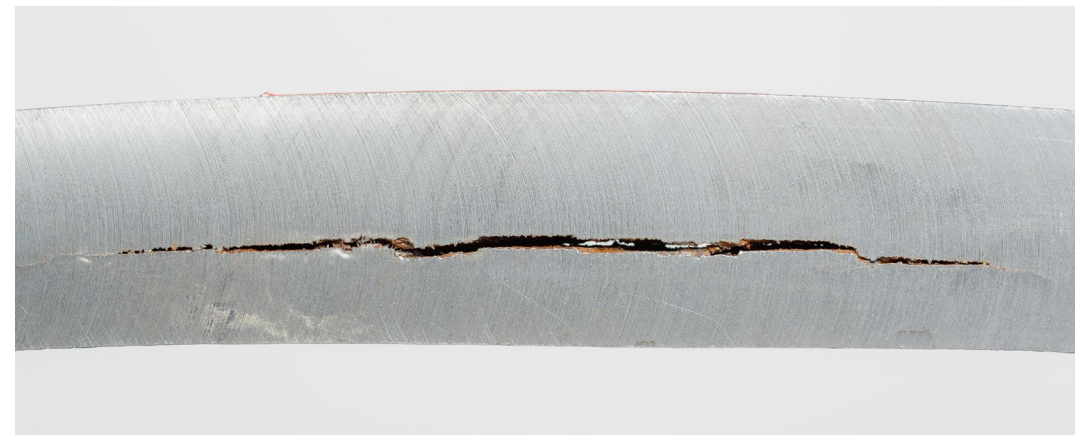
Hydrogen-induced cracking in metal. Photo by CEphoto, Uwe Aranas.
