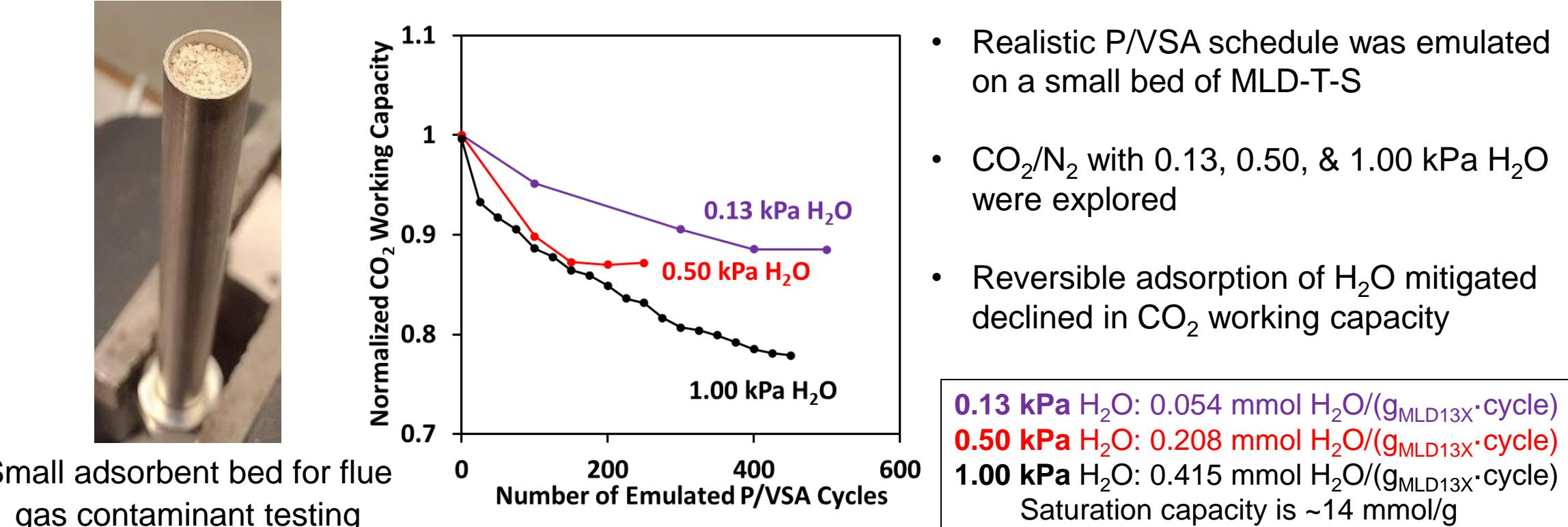
Note: MLD-T-S can be fully regenerated at 200°C.
