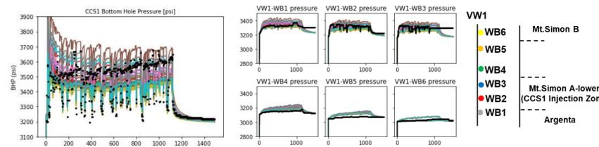
Figure 3. Observed (black) and Eclipse simulations-based (color) daily bottom hole pressure data at the CCS1 injection well (left) and multi-depth sensors at a verification well (VW1).
