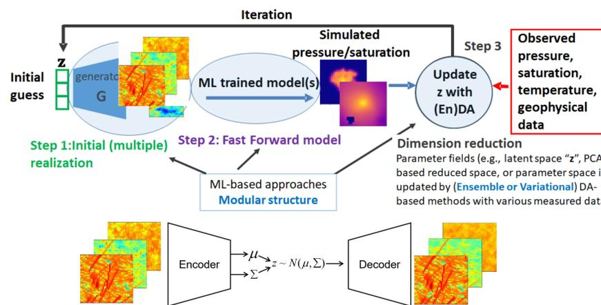
Figure 1. (top) A schematic of latent space-based data assimilation (LSDA) with ML forward models and (bottom) variational autoencoder for 3D permeability, porosity, and fault transmissivity multipliers.
