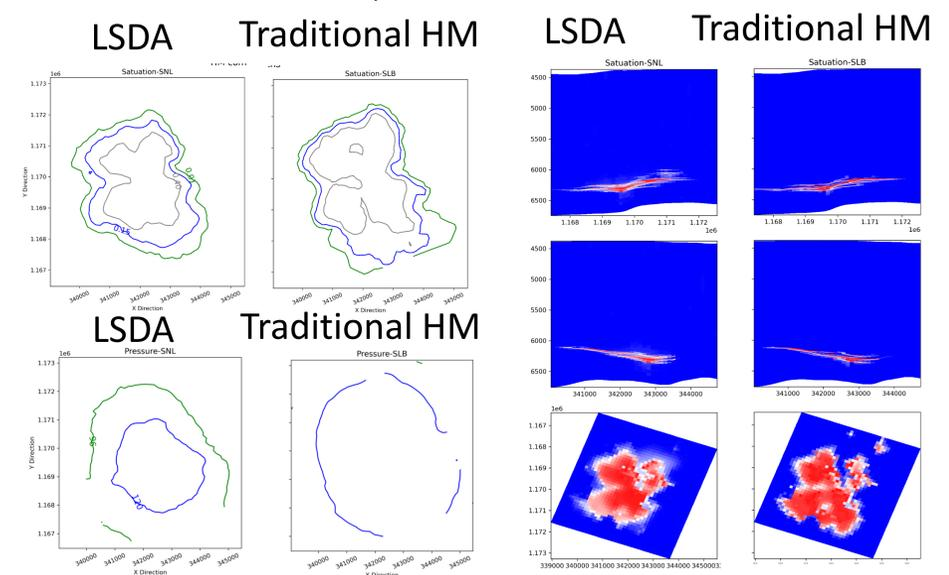
Figure 8. Area of review comparison for CO<sub>2</sub> saturation (top) and pressure (bottom) as well as CO<sub>2</sub> plume distribution (right)..
