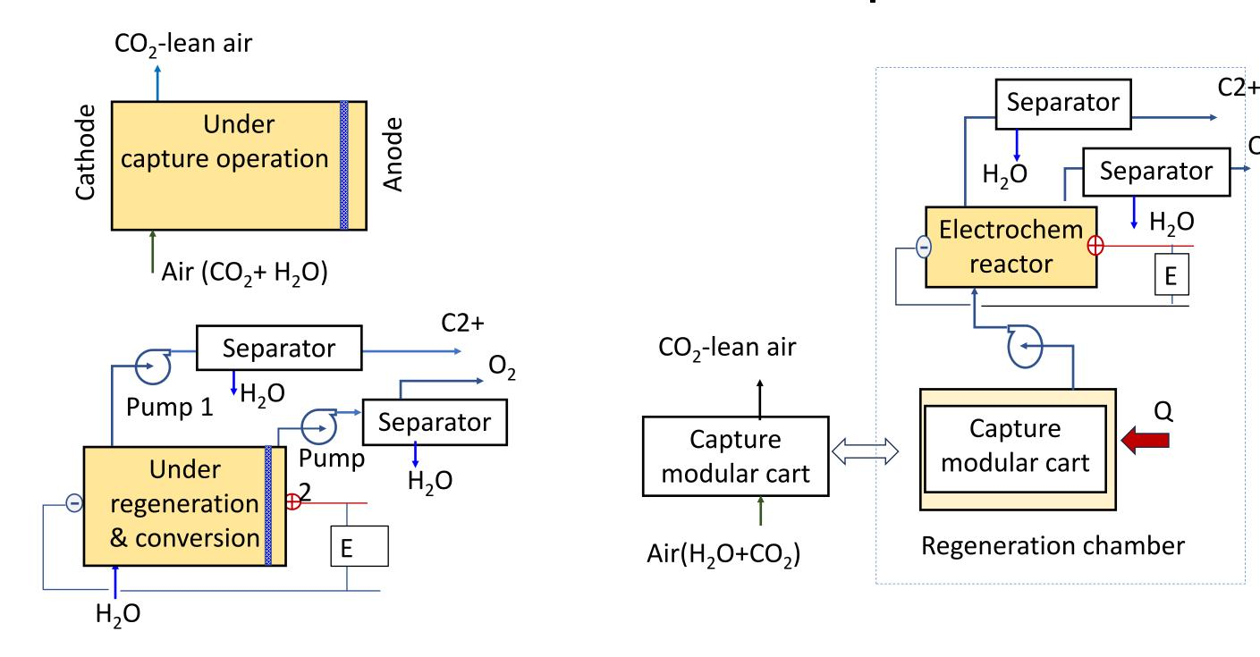
Molecule Works' adsorption/heat exchange (AHX) reactor designs for direct air capture with low cost and low energy consumption
