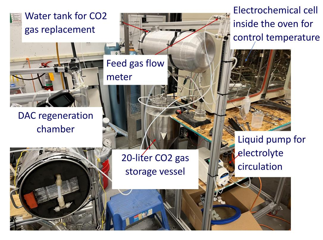
>95% CO<sub>2</sub> can be produced by regenerating the adsorbent with hot water heating and rough vacuum pulling
