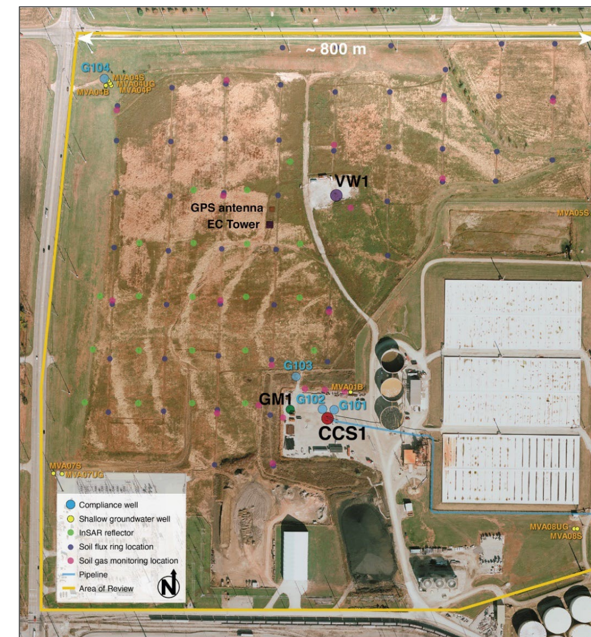
Map of the IBDP storage project showing locations of wells and near-surface monitoring equipment
