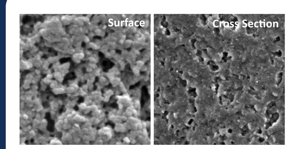
Preliminary data and analysis revealed similar porosity between the surface and internal structure of the candidate RGTM.
