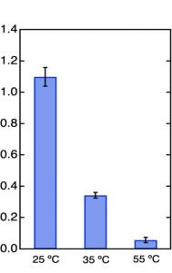
• Humidity enhances the CO<sub>2</sub> capacity and amine efficiency of the PEI, due to increased mobility and facilitated carbamate formation. Enhancement due to humidity decreases with temperature due to decrease in overall water
