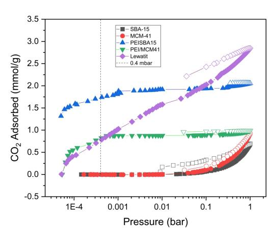
Representative excess pure CO<sub>2</sub> sorption isotherms at 25 °C (298 K) for various DAC materials. The dotted line marks CO<sub>2</sub> uptake at 0.4 mbar (equivalent partial pressure to 400 ppm). Filled symbols are for adsorption; open symbols are for desorption. Uptake is given as mmol of  $CO_2$  per g of dry sample.
