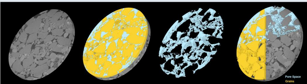
Example of segmentation from grayscale three-dimensional (3D) CT image: matrix grains in yellow, and pore space in pale blue.
