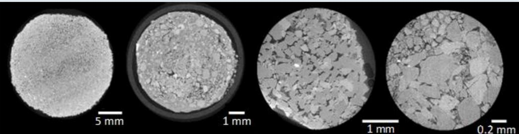
Two-dimensional (2D) slices through a selection of CT scans of Mt. Simon Sandstone cores. Leftmost image is from a lower resolution (14.79 μm) scan from the Industrial CT scanner, while the remaining images showcase the range of higher resolutions possible with the Micro-CT scanner.
