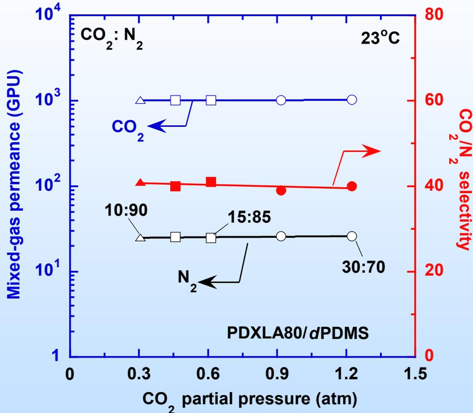
**CO<sub>2</sub> permeance and selectivity are independent of CO<sub>2</sub> partial pressure**
