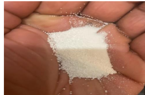
Matrix with 50% w/w NaOH solvent and metallic oxide solid adsorbent. Resulting composite is safe to handle.
