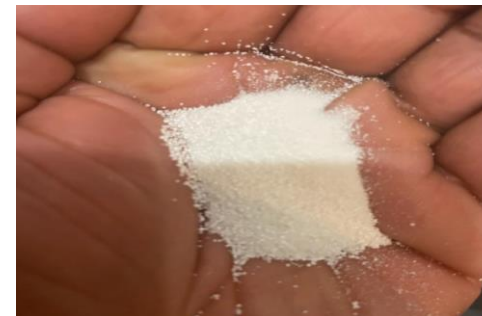
Matrix with 50% w/w NaOH solvent. Resulting composite is safe to handle.
