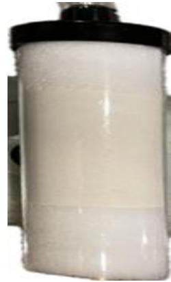
Sample composite matrix with Amine + Metallic Oxide - 8 gm CO 2 captured in 50 mL matrix*
