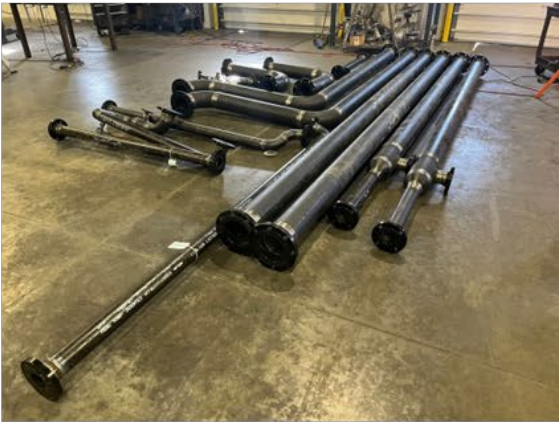
Large bore CS piping
