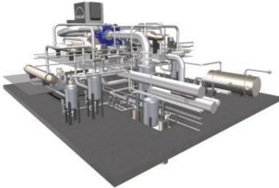
Illustration Of compressor train with integrated Carbon Capture Heat Recovery (CCWHR) technology (Image courtesy of MAN Energy Solutions)
