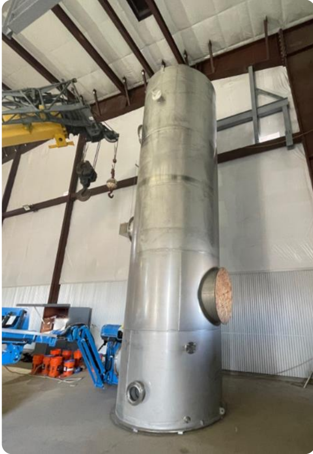
Direct Contact Cooler - Feb
