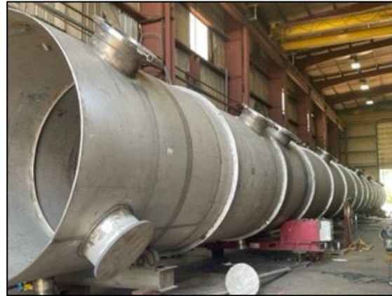
Columns at fabricator shop
