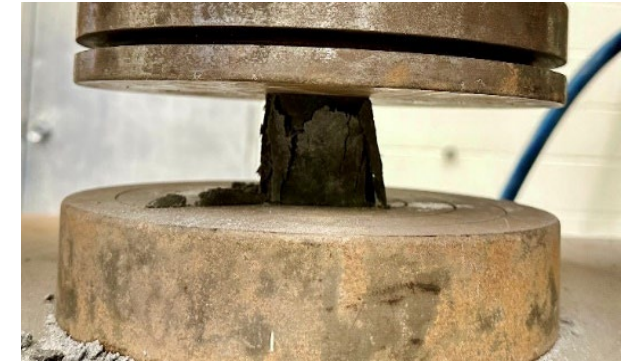
Compressive strength testing
