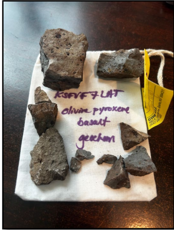
(1) Samples split for reactivity, whole rock geochemistry, thin section
