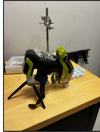
(3) Rock and powdered samples analyzed with Niton XL5 portable XRF (pXRF) then sent to a lab for pressed pellet XRF/ ICPMS/ ICPOES
