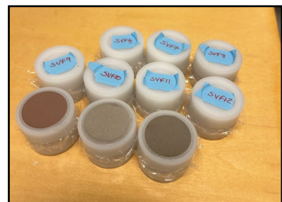
(2) Reactivity samples crushed, powdered, homogenized, & sieved to <63 microns
