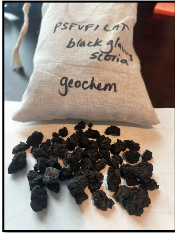
(1) Samples split for reactivity, whole rock geochemistry, thin section
