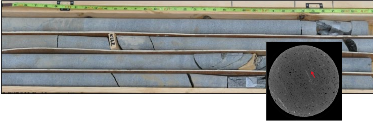
Figure 75: 2D image from industrial CT scan of the Susquehanna River core at 129.2 ft. where the red arrow indicates a mineralized fracture.
