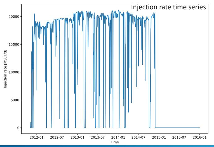
Operational injection started on Nov 17<sup>th</sup>,2011 and was completed successfully on Nov 26<sup>th</sup>, 2014 with a total volume of 999,231 tons.
