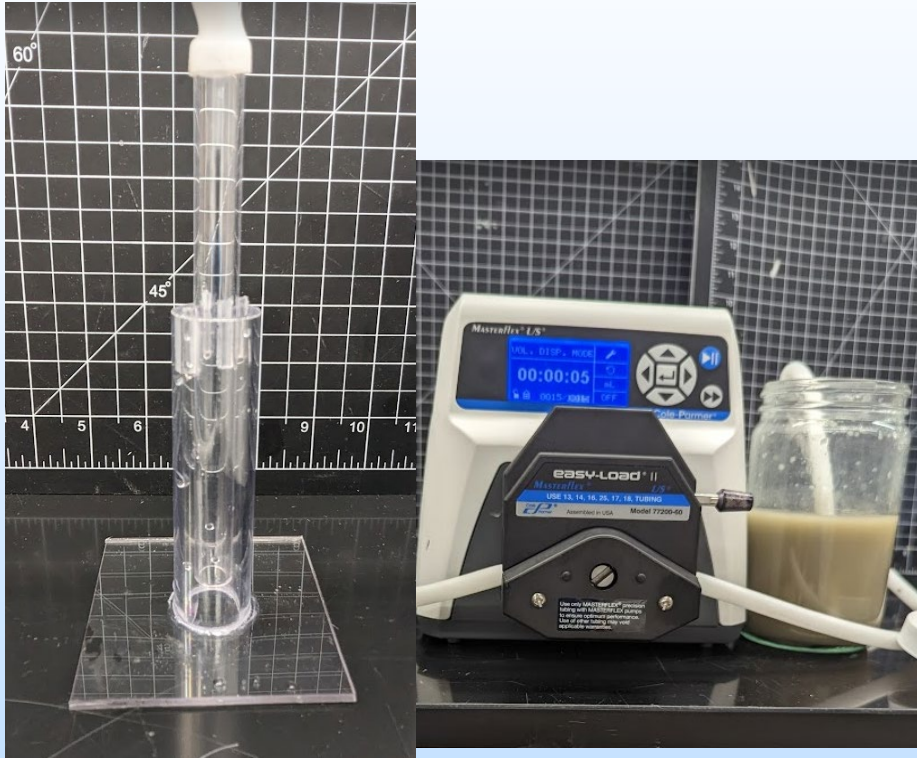
Peristaltic pump to pump cement in a mock wellbore
