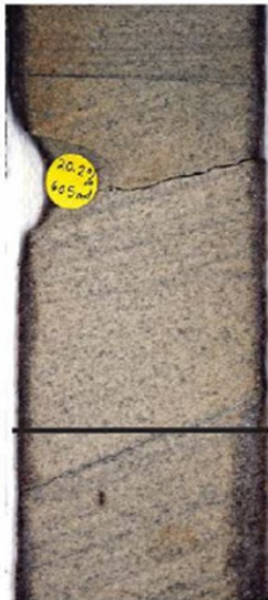
Well D-9-8 #2 at 9,449 ft. showing planar cross-bedded sandstone.
