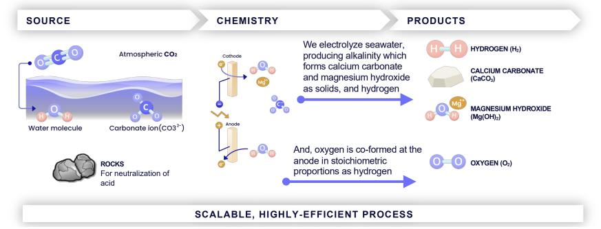
~2.3 MWh per tonne of CO<sub>2</sub> removal is the lowest demand for atmospheric CDR
