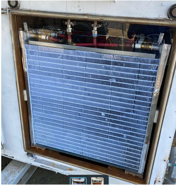
Radiators coated with P/TSA MOF
