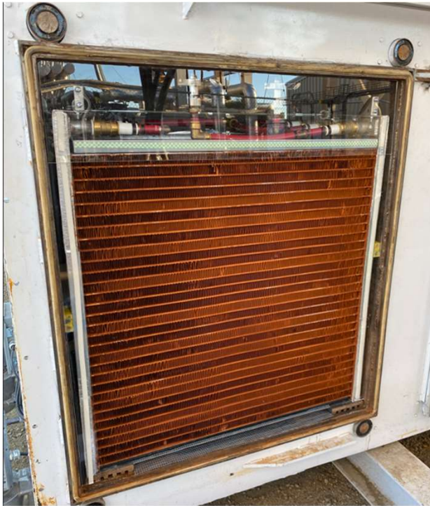
AWE radiators coated with dessicant MOF
