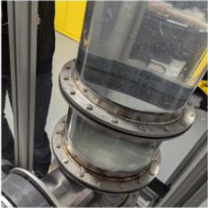
Air-contactor column filled with liquid
