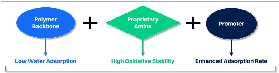
Macroporous polymer backbone for reduced water adsorption
