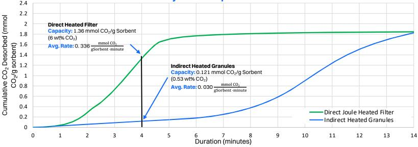
Direct Joule heated filter shows 10x increase in desorption rate - can achieve performance targets
