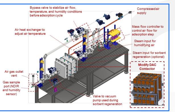
Modify existing bench system to incorporate new contactor design Finalizing design with the filter vendor
