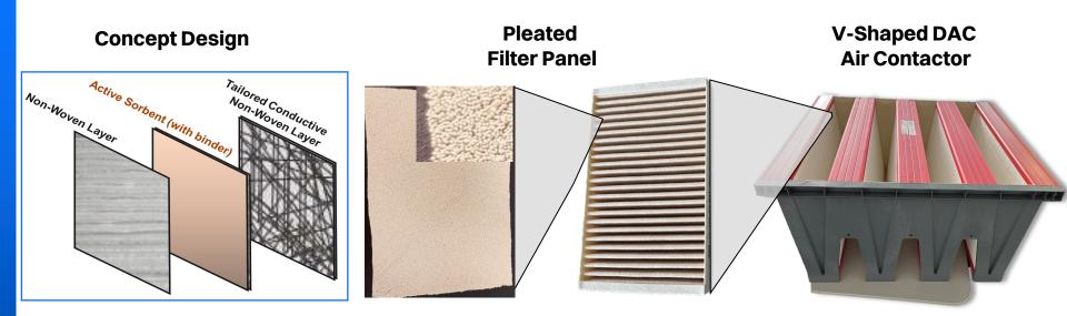
Electrically conductive structured sorbent filter assembly Nonwoven filter with sorbent (ECCOsorb 1). Up to 1.2 kg sorbent/m<sup>2</sup> loading 24"x24"x12" Size module capable of holding up to **10 m<sup>2</sup>** of sorbent surface area
