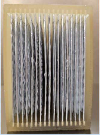
3d-printed laminate module to accommodate 3" height -6" length laminate sheets
