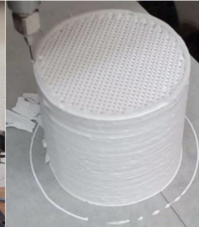
4" x 8" 3D printed ceramic monolith
