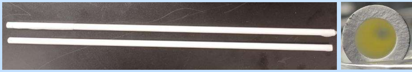
Na + - nanochannel ceramic hollow fiber membrane
