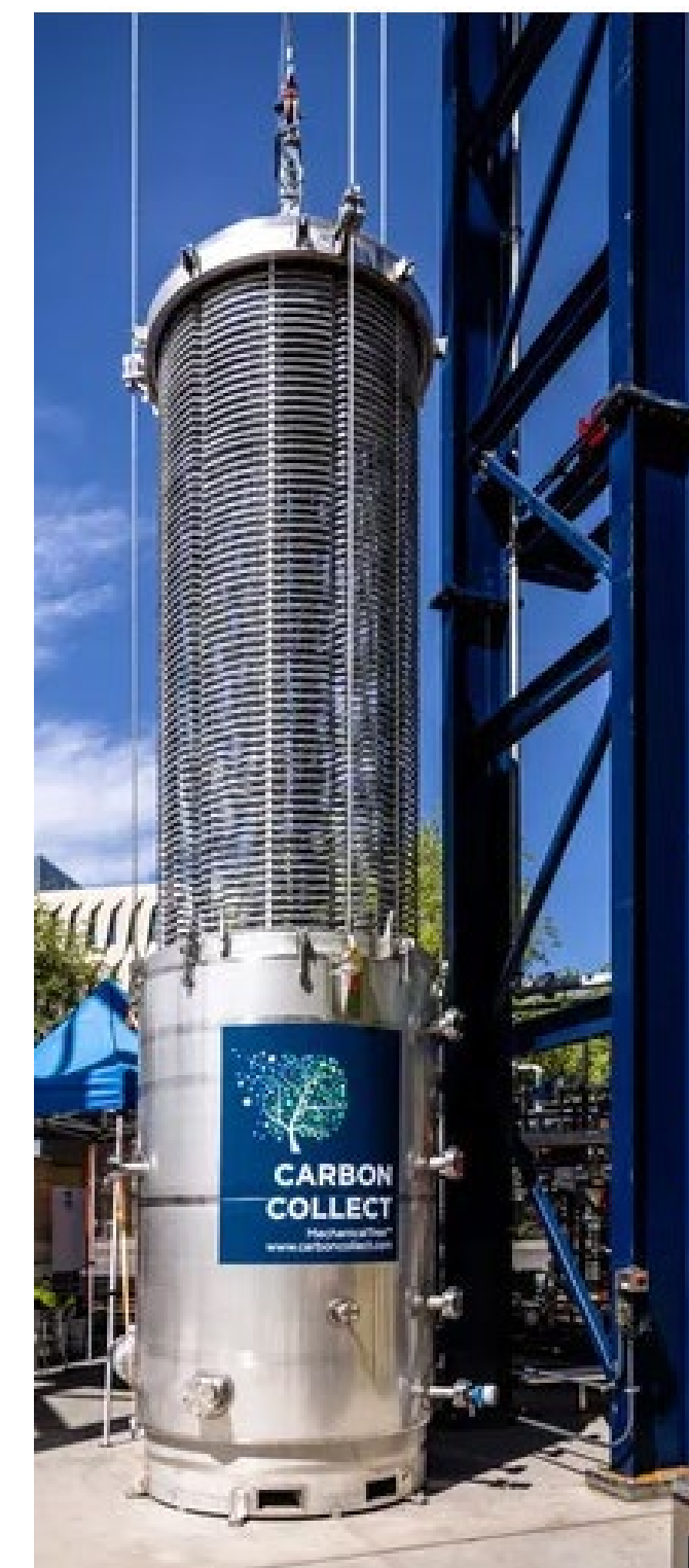
Carbon Collect Inc. MechanicalTree™ installed at ASU passively collects CO 2 delivered by the wind from any direction with a low pressure drop.
