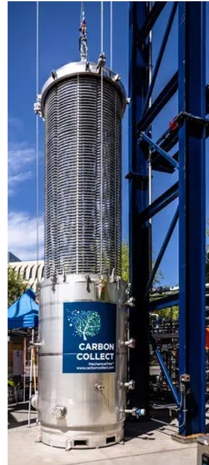
Carbon Collect Inc. carbon tree installed at ASU
