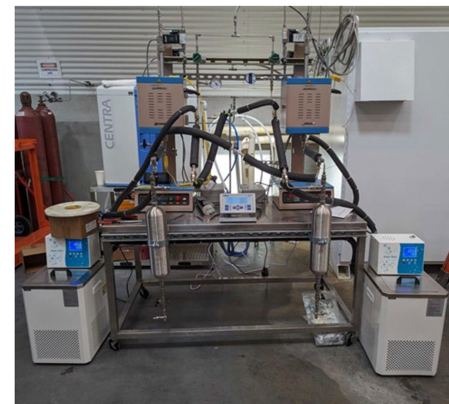
Air Company bench-scale CO 2 to fuels reactor system (for Phase II).
