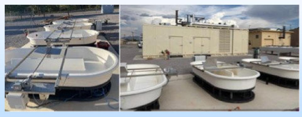
Strain Testing in Outdoor Ponds Carbon Utilization Efficiency MBE Ponds with NMSU Ponds with traditional diffusers novel saturator system pH 7.5-8.0 not determined pH 7.5-8.0 <40% pH 8.5-9.0 50-55% pH 8.5-9.0 60-90%
